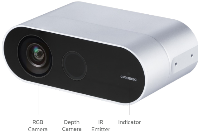
Femto Bolt front view showing components
