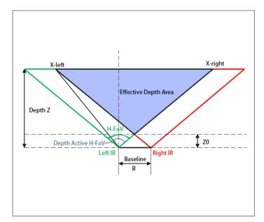
Depth Field of View (Depth FOV) at any distance (Z) can be calculated using the following equation:
